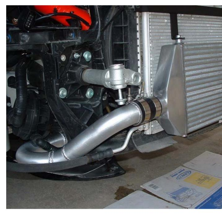
5) Locate the by-pass-valve bung on the passenger side pipe. Depending on the type of by-pass-valve your vehicle is setup with will determine if the provided 90 degree needs to be trimmed. The by-pass-valve hose will look exactly as pictured if your vehicle is using the stock valve. See picture below.
