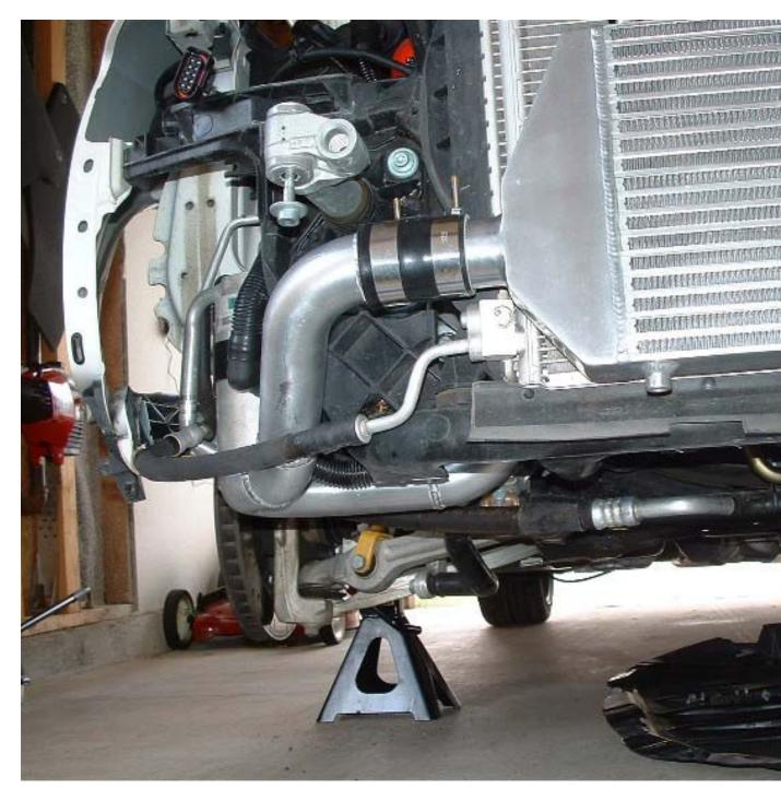
7) Install the boost sensor on the driver side pipe.
