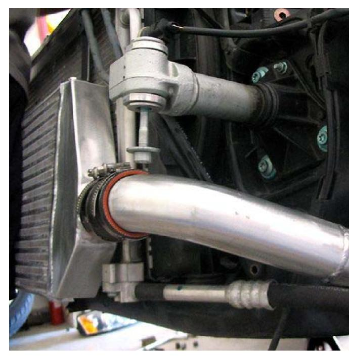
8) Double check all t-bolt clamps and intercooler alignment. Reverse install the bumper , headlamps, and belly pan.
